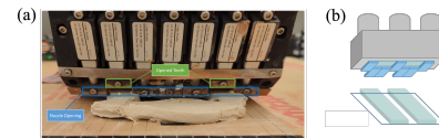
Fig. 5. (a) SSE variable-geometry outlet, (b) Integrated architecture: multi-inlet paired with the Selective Sheet Extrusion (SSE) system
