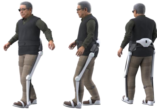
Fig. 1. Concept design of a wearable robot for elderly users and individuals with lower-limb paralysis.
