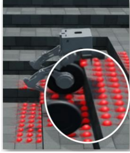
Figure3. Contact-trigger activation during wheel-stair interaction.
