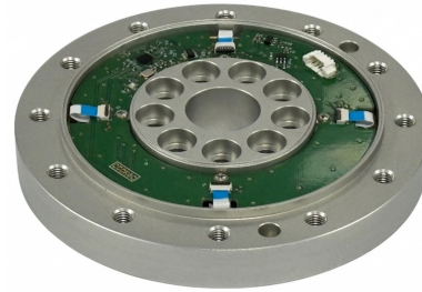
Fig. 4. Prototype of the developed high-stiffness joint torque sensor.
