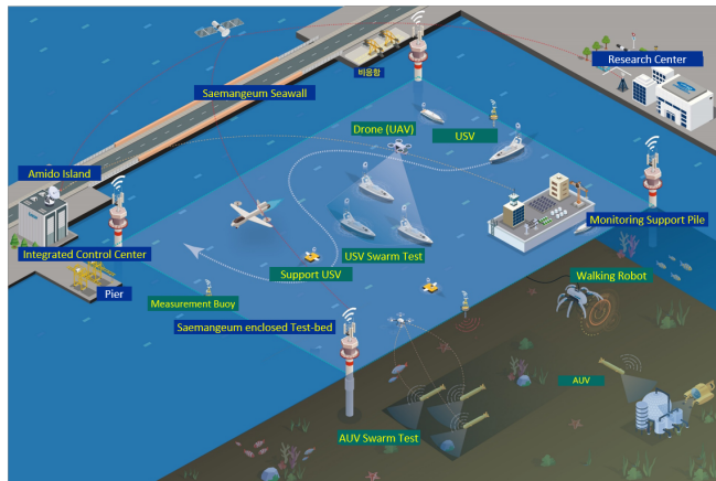
Fig. 1. Conceptual illustration of the Saemangeum enclosed-sea test site. The testbed supports multi-domain unmanned systems including USVs, AUVs, and UAVs, along with measurement infrastructure and integrated control systems.
