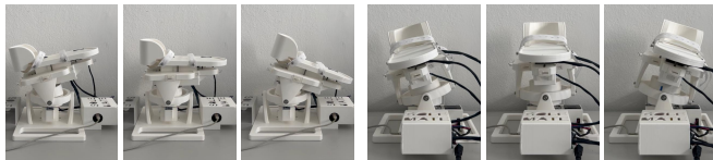
(a) Lateral view of dorsiflexion/plantarflexion (D/P) motion. (b) Frontal view of inversion/eversion (I/E) motion.
