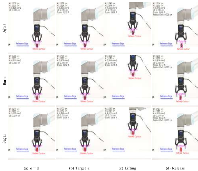
Fig. 1: Grasping sequences for Ajwa (7%), Barhi (7%), Sagai (5%): (a) zero-strain contact, (b) bioyield strain, (c) 30 cm vertical lift, (d) post-release recovery. All fruits returned to original geometry with \delta_r < 1 mm.
