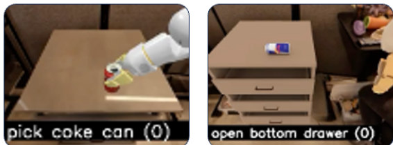
Fig. 3. Example simulation environments from SimplerEnv Fractal. (Left) Pick coke can — a simple single-object grasping task achieving 90% success rate. (Right) Open bottom drawer — a complex articulated manipulation task achieving 10% success rate. The stark visual and performance contrast illustrates the challenge gap that imitation learning alone cannot bridge.
