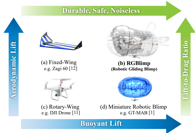
Fig. 1. The schematic of the conceptual design of the RGBlimp inspired from existing miniature aerial vehicles. While with advantages in buoyant lift, robotic blimps (d) are more durable, safer, and less noisy, their aerodynamic performance is rarely considered. In contrast, fixed-wing gliders (a) are designed to take advantage of the gliding mechanism with a higher lift-to-drag ratio but generally lose aerodynamic efficiency at low speed. Combining the advantages of buoyant and aerodynamic lift, the RGBlimp (b) as a hybrid aerial robot is designed to adapt to low-speed flight with improved aerodynamic performance.
