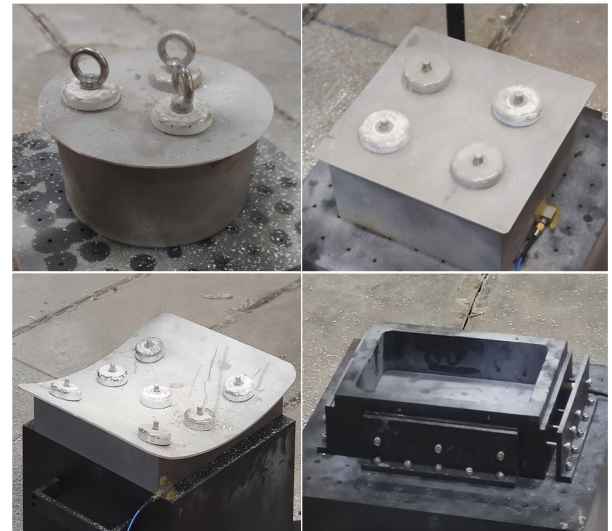
Fig. 13. Four types of workpiece sample are selected to be machined, including square plane sample, circular plane sample, curved aircraft skin sample, and cavity sample.
