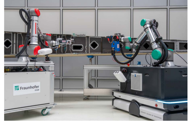
Fig. 1. Fraunhofer IFAM develops a multirobot assembly system for manufacturing a lighter aircraft fuselage of the future made of thermoplastic fiber-reinforced plastics (FRP) [6].
