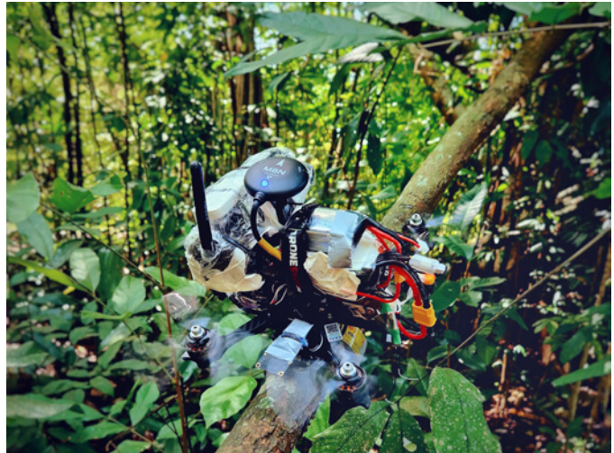
Fig. 1: Agile quadrotor perching on tree branches of steep incline during XPRIZE Rainforest semifinals, Singapore 2023.
