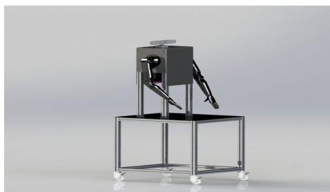
Fig. 3. The developed dual-arm robot for human-robot collaboration
