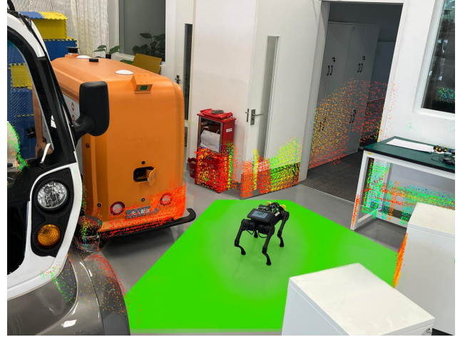
Fig. 1. Overview of the proposed methodology. The proposed reactive controller aims to minimize the tracking error while constraining the robot with specific geometry inside the free region (shown in green) by solving a constrained polynomial optimization problem with safety-related polynomial no-negativity constraints.
