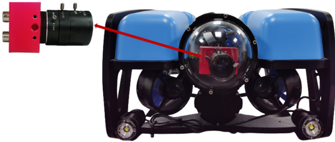
Fig. 2. (Left) Event camera. (Right) ROV equipped with an event camera.
