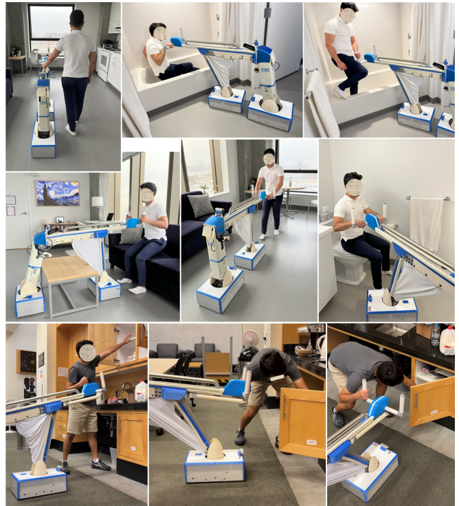
Fig. 9. Use cases: demonstration of the 2BB providing assistance with common activities of daily living. From left to right, the first row shows ambulation in a corridor, standing up in a bathtub, and stepping over a bathtub lip onto a slippery floor. Row 2 demonstrates standing up from a couch, using the robot as a walker, and sit-to-stand from a toilet. Row 3 demonstrates reaching up to grab an item from a shelf, and reaching down to grab an item from a drawer (shown from two different angles).
