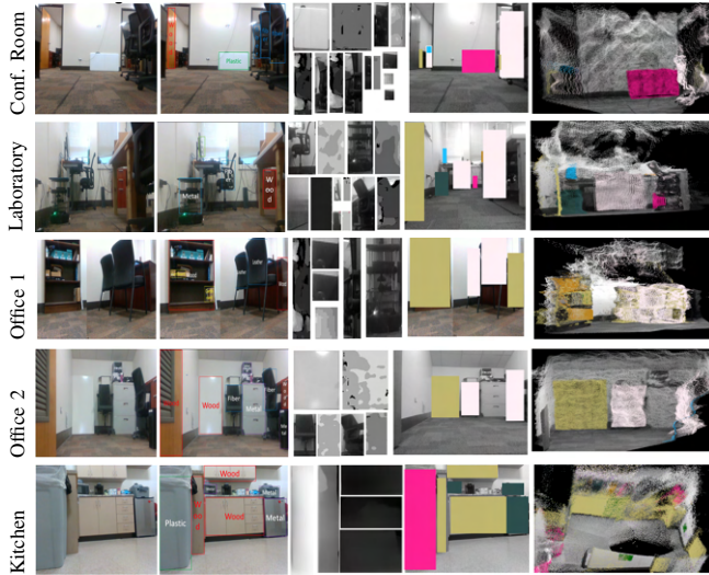
Fig. 5: Demonstration of sample outputs at various stages in our pipeline for the real-world robot RGB-D datasets. From left: RGB Image, ground truth material labels, segmented objects, material classification, and the final 3D clustering.
