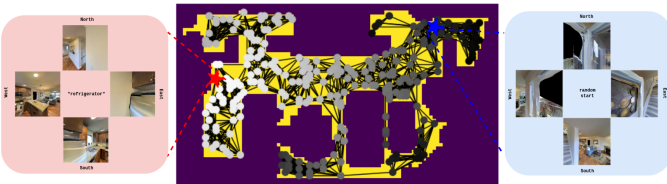
Fig. 7: Visualization of our navigation environment. On the left, we show the constructed geometric graph in an HM3DSem scene. The density of color represents the distance to the goal. On the right, we demonstrate the observation example on each node, which consists of four egocentric RGB images facing four directions.
