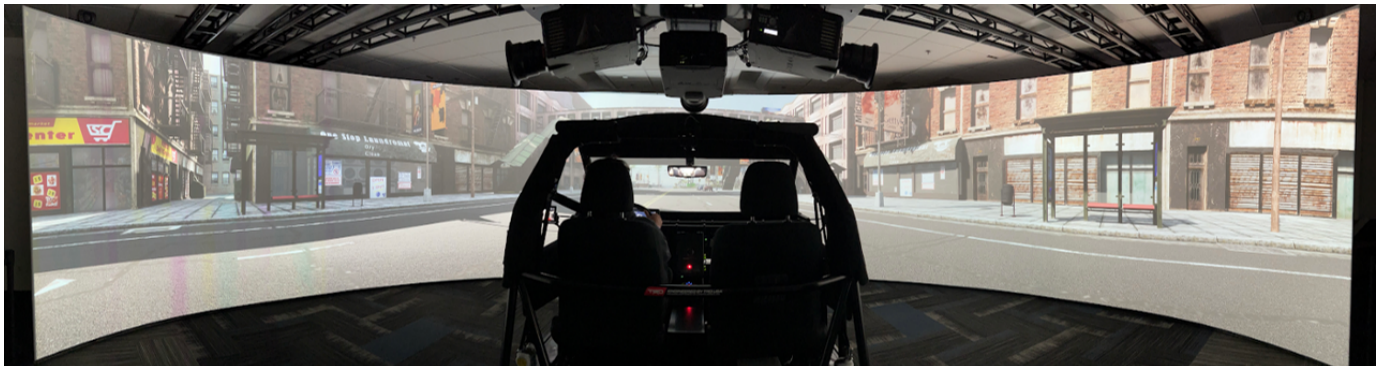
Fig. 1: This figure shows the 6-DOF driving simulator that we employ in our study. Using this simulator, we demonstrate that MAVERIC is capable of mimicking driving style as well as modulating the level of aggression. Additionally, we show that personality, perceived similarity, and high-velocity driving style impact the effect of homophily.
