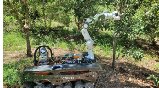
Fig. 1: Autonomous navigation task: Our field robot obstructed by vegetation.
