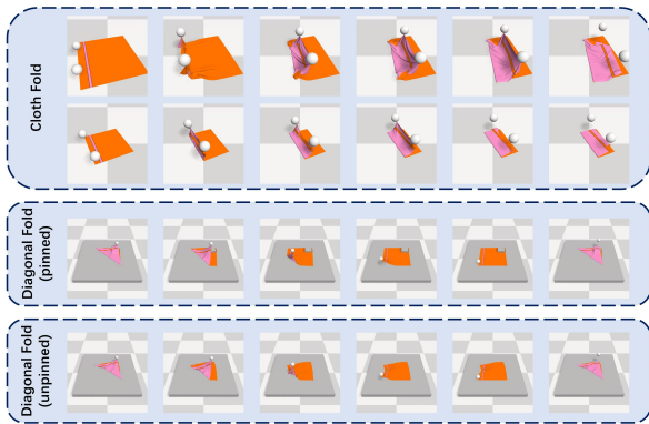
Fig. 5. Snapshots of the proposed method. We evaluate our proposed methods by adopting three cloth manipulation tasks. Only image observation is used for the agent to generate trajectory. More demonstration can be found in the multi-media resource.
