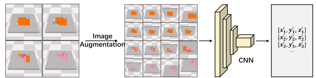
Fig. 3. CNN Model: We design a CNN encoder to estimate the state information from image observation. Image augmentation is applied to improve the robustness of state estimation.
