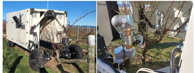
Fig. 1: Archie Jnr in the vineyard driving over the row of vines on the left, and the internal view of the robot platform with the side panels removed on the right.
