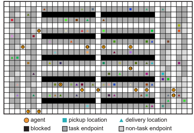
Fig. 3. Four-neighbor grid environment [9]. A pair of pickup and delivery locations with the same color represents a single task. In MAPD-D, each delivery location is assigned a deadline.
