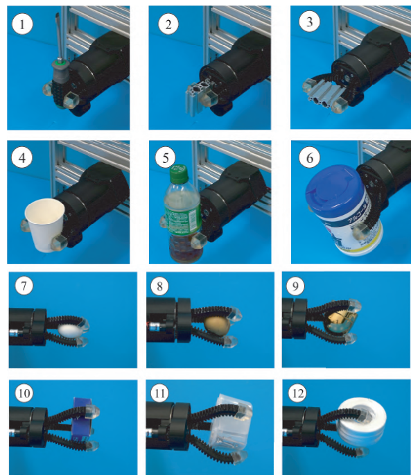
Fig. 15. Grasping experiments of two and three-fingered gripper.
