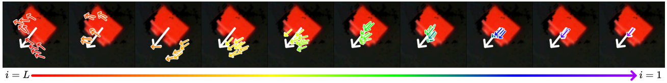
Fig. 2: An illustration of the iterative refinement of pose estimates through denoising steps. White arrows represent the ground truth, while multi-colored arrows, transitioning from i = L to i = 1 , signify the evolving pose estimate at each step.
