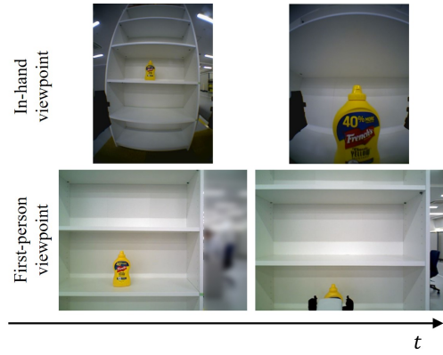
Fig. 9. Visual observations in the pick-bottle-from-shelf task. Figures are lined in time-step order from left to right.
