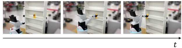
Fig. 5. Overview of the pick-bottle-from-shelf task. Figures are lined in time-step order from left to right. Left: the MM started with o_h and o_f facing the bottle placed on the shelf. Middle: the MM moved the mobile base and arm to reach the bottle. Right: the MM picked up the bottle from the shelf.
