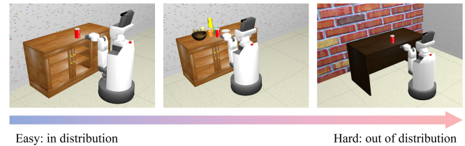
Fig. 2. Example of visual observation domain shift. Left: environments for training the policy. Middle: distractor objects cause the minor change. Right: unknown furniture causes the major change.
