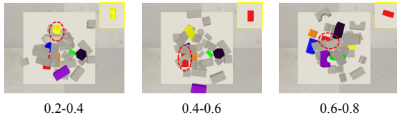
Fig. 6. Examples of different occlusion ratio cases in simulation . These three cases represent occlusion ratios of 0.2-0.4 (left, yellow block), 0.4-0.6 (center, red block), 0.6-0.8 (right, red block), respectively. They are randomly selected from blocks that meet the requirements of the occlusion ratio.
