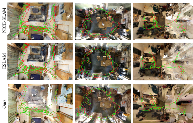
Fig. 3: Qualitative Comparison on ScanNet. The ground-truth camera trajectory is shown in green and the estimated trajectory is shown in red. Our method predicts more accurate camera trajectories and does not suffer from pose drifting.
