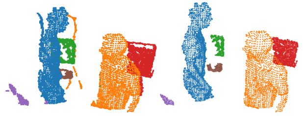
Fig. 3: Outlier removal with semantic perception on point clouds, resulting in unchanged dynamic interpretations based solely on RGB images.
