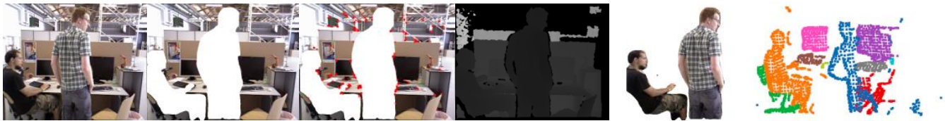
Fig. 2: Segmentation of hypothesized moving objects with keypoints on static objects and background, and point clouds of object instances.
