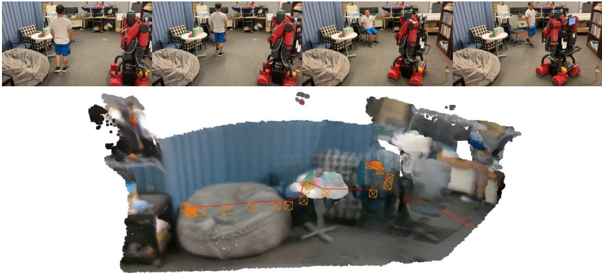
Fig. 6: Moving sequences of the Baxter robot (top) and the resulting reconstructed 3D scene with the estimated camera trajectory (down). The red line indicates the estimated camera trajectory with optimization, and orange frustums mark camera poses along the trajectory.
