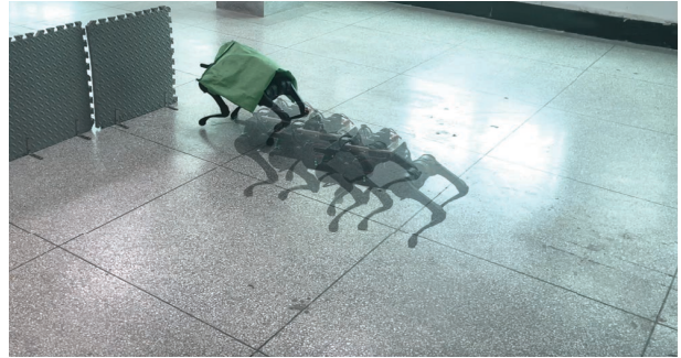
Fig. 1. The navigation application with KLILo. During the navigation, the shade cloth is put onto the robot, such that the LiDAR points become ineffective.
