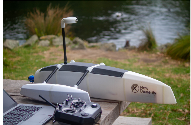
Fig. 1: The proposed autonomous, 3D printed, waterjet-powered, open-source robotic trimaran.
