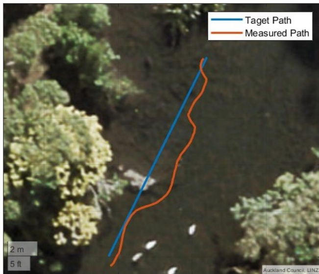
Fig. 10: Obstacle avoidance of rocks located in the Western Springs lake in Auckland, New Zealand ( 36^{\circ}51'55.7''S , 174^{\circ}43'19.6''E ) using the 'bendy-ruler' algorithm from the 2D LiDAR data.
