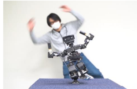
Figure 1. EVAL-03 imitating human motion
