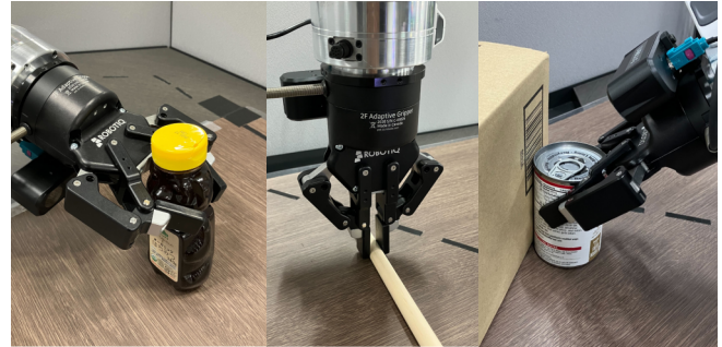
Fig. 1. While existing works only handle precision grasping, power grasping is more robust against both initial position error and post-grasp force disturbance. We propose a data generation pipeline and neural network model that prioritizes power grasping if applicable (left) but implicitly switches back to precision grasping if power grasping is not available due to collision with the table (middle) or other objects (right.)
