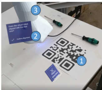
Fig. 3. (1) A QR code and (2) textual instructions were used to calibrate and (3) align the cobot with its model to ensure correct robot tracking [5].
