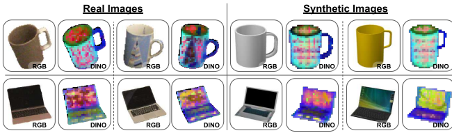
Fig. 3. Semantic Features: DINOv2 features via 3-dimensional PCA with input RGB to understand the consistency across the different instances.
