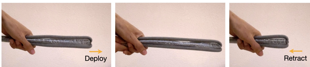
Fig. 10. Solid-state vine robot comprised of foam rods everting through bending, which removes the need for inflation
