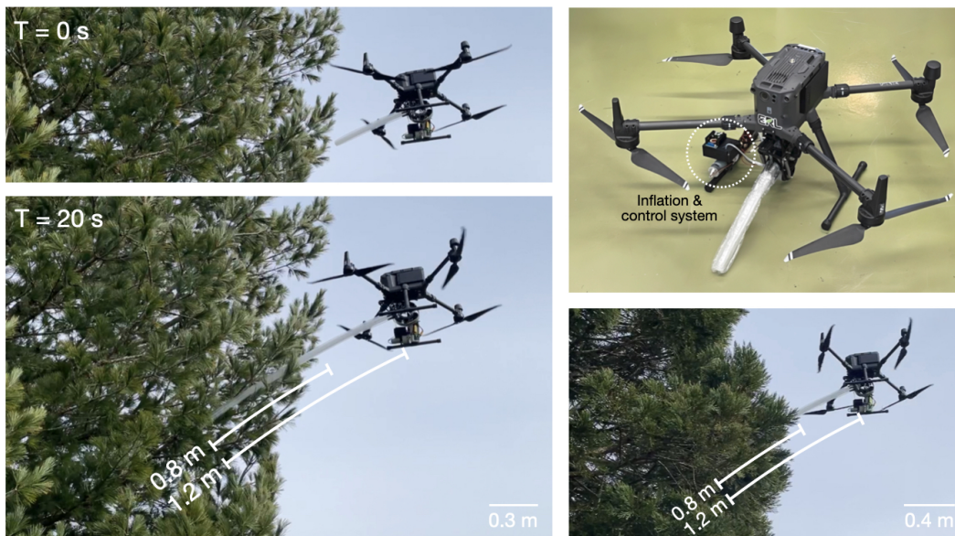
Fig. 9. Drone-based cantilevered vine robot with potential applications in environmental DNA (eDNA) sampling from inner tree canopies, demonstrated by deployment into a pine tree ( Pinus peuce ) (left) and a cypress tree ( Sequoioideae ) (lower right), the demonstration system (upper right)
