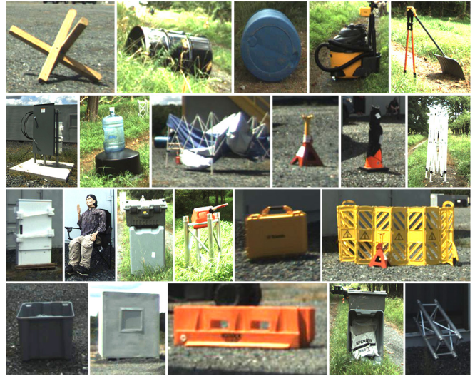
Fig. 6. Subset of obstacles included in the AvOID dataset. The obstacles are cropped from the original RGB images for the presentation purpose only.
