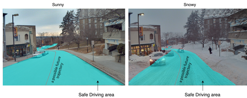
Fig. 1 This example from the Ithaca365 dataset [8] shows the drivable area ( i.e. , potential trajectory choices) shrinks with the degradation of weather conditions (sunny \rightarrow snowy). The blue overlay indicates the safe driving area. The red curved line indicates a possible future trajectory for the agent.
