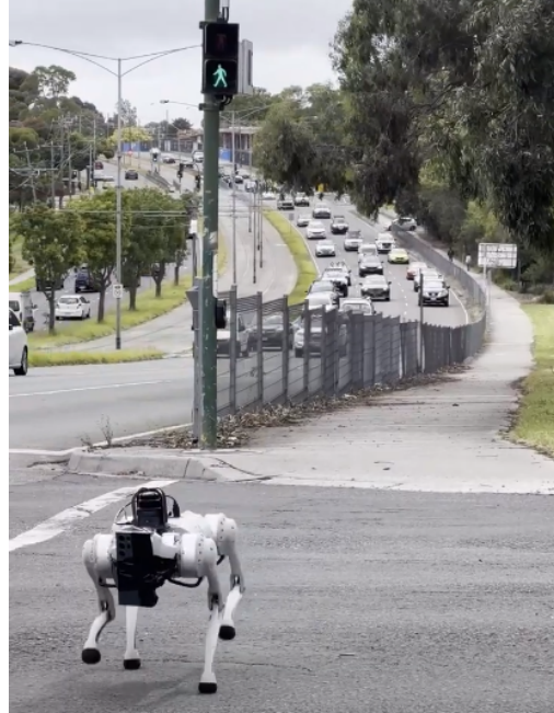
Fig. 1: In urban settings, robots often struggle with visual occlusion, hindering their ability to detect traffic lights. Our solution combines auditory cues with vision, utilizing traffic lights’ sound patterns to indicate their state. This method ensures robots can navigate effectively, even when visual signals are obscured.
