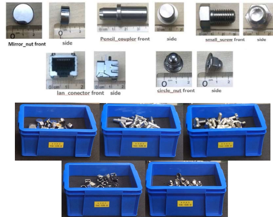
Fig 10 . Top: the 5 different target objects with shiny surfaces and different shapes. Bottom: 20 piled target objects in each box (50cm*25cm) for picking experiments.
