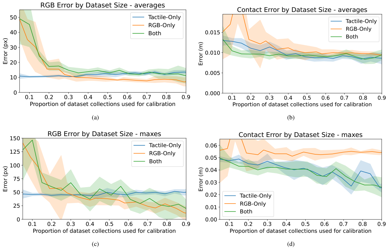
Fig. 5. Line plots illustrating (a) average RGB errors, (b) maximum RGB errors, (c) average tactile errors, and (d) maximum tactile errors when calibrating across different modalities. The results show the average of 10 runs, with the standard deviation presented in an error bar.
