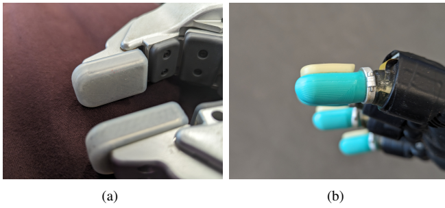
Fig. 2. Tactile sensors used for contact detections: (a) PR2 fingertip pressure sensors; (b) SynTouch BioTac mounted on the fingertips of the Shadow Dexterous Hand.
