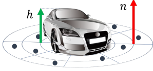
Fig. 4: Semantic-based height estimation. We harness the points with ground semantic in descriptor to estimate the camera height relative to the current ground plane.
