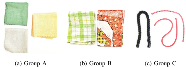
Fig. 4: The sets of deformable objects employed in the experiments consist of three uniform-colored soft clothes, two textured soft clothes, and three ropes with different textures and diameters.
