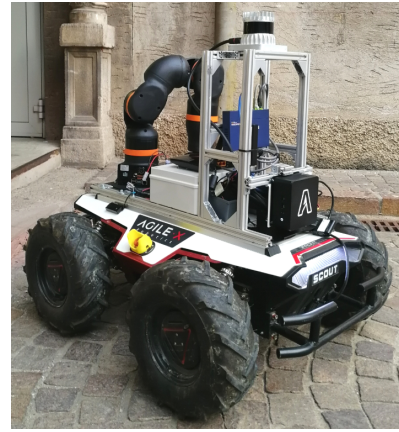
Fig. 2. Robot used to test the generated behavior trees
