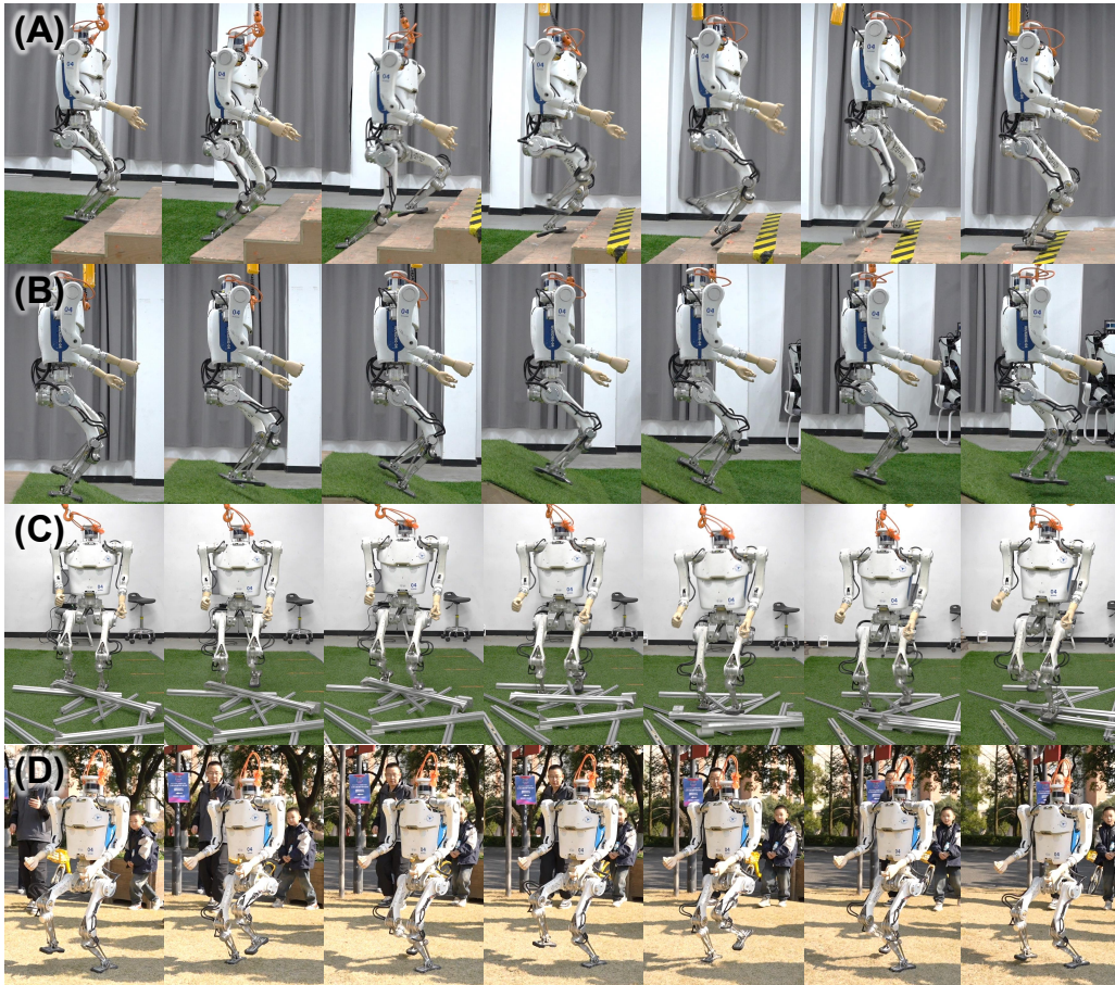
Fig. 7: Snapshots of Wukong-IV humanoid traversing different terrains. (A) 3-step 10cm stairs. (B) 25 deg slope. (C) Indoor terrain with aluminum profiles. (D) Natural grass field. Check the supplementary video for more experiments.
