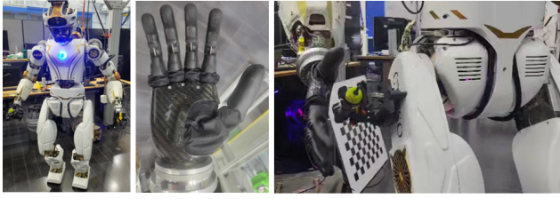
Fig. 2: NASA Johnson Space Center’s Valkyrie robot (left) with the PSYONIC Ability Hand mounted (center) and a tool holster on the right hip (right).
