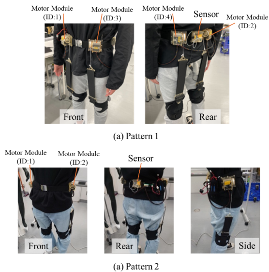
Fig. 5. The appearance of the developed modular robot wear. (a) Sagittal plane assist. (b) Frontal plane assist.
