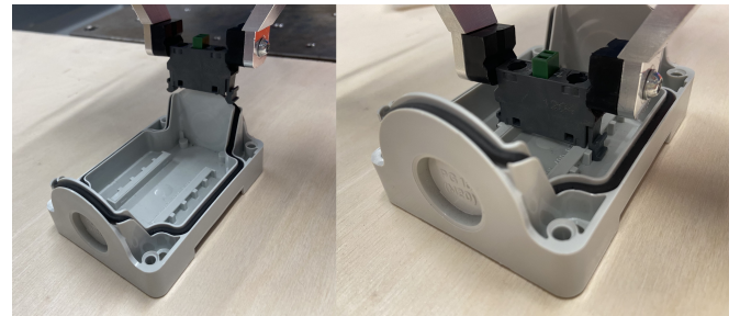
Fig. 9. Comparison between the final position of the switch before iterative learning was used (left) and after eight iterations of the proposed learning controller (right) for the snap-fit assembly of a switch.
