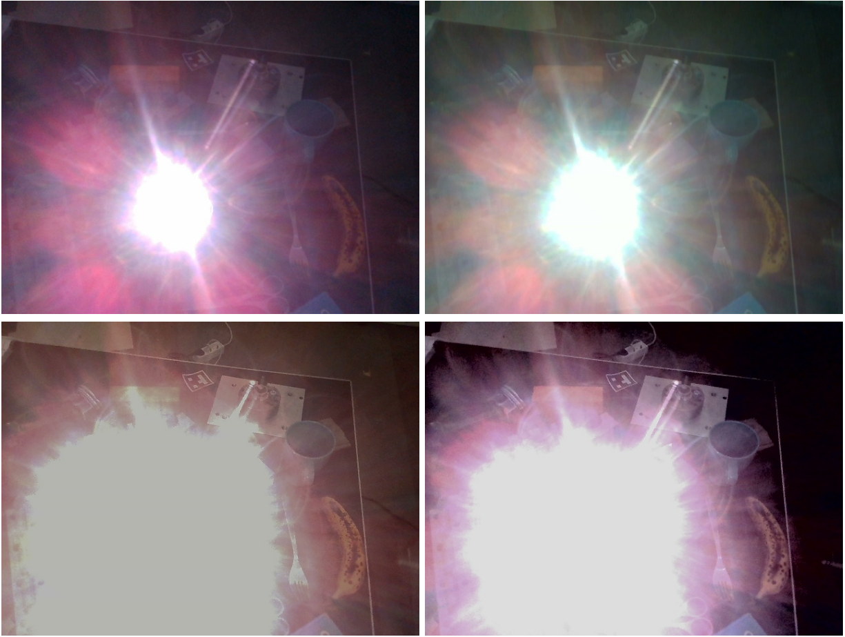
Fig. 5. Example images captured during experiments. Top left: default parameters. Top right: Default parameters with auto-exposure and auto-whitebalance. Bottom left: parameters optimized according to [3]. Bottom right: parameters optimized using our NF gradient image.
