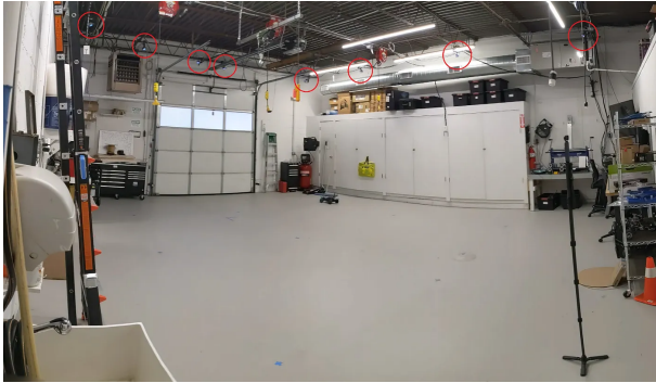
Fig. 2. Our test garage where 12 OptiTrack Prime 13 cameras are mounted on the ceiling. The cement floor in this garage is used for pre-training of a learned model.
