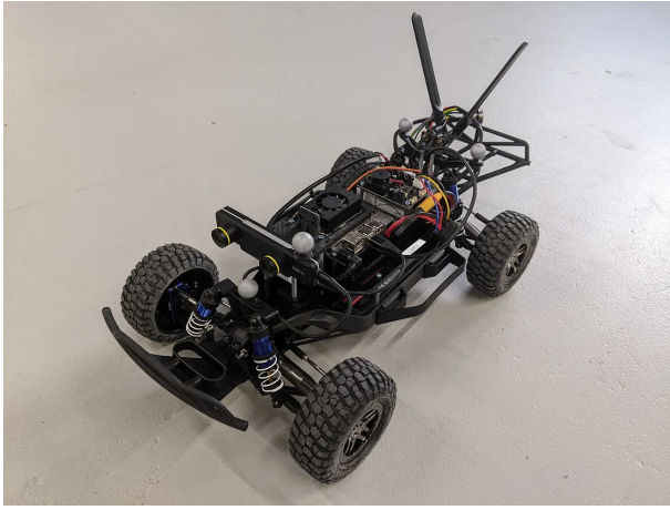
Fig. 1. TRIKart, a one-tenth scale-car which is used for our experiment. During experiments, electrical devices are covered by a plastic body and a bumper is mounted around the perimeter.
