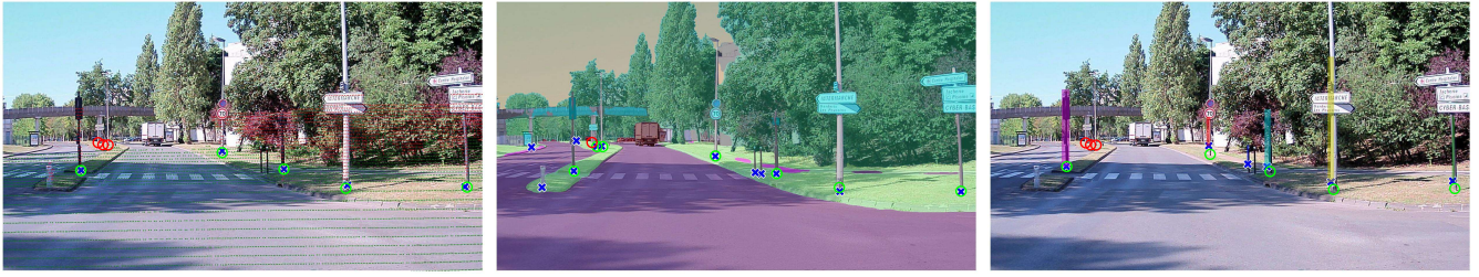
(a) M annotation using the map with lidar (point-cloud in green for ground). (b) S annotation overlaid with the segmentation mask. (c) L annotation with projected lidar clusters.
